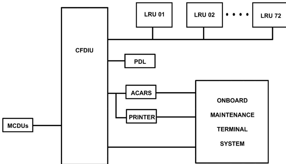
FIGURE 31.9 MD-11 maintenance system architecture.
