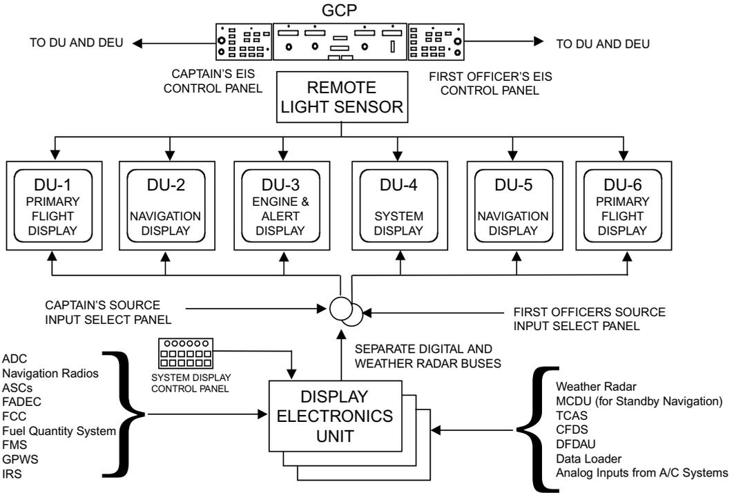
FIGURE 31.6 Display system architecture.
