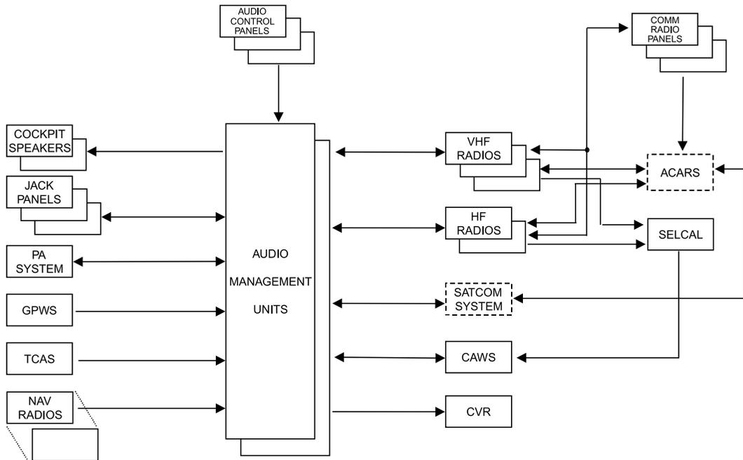
**FIGURE 31.4** Communication system architecture.
