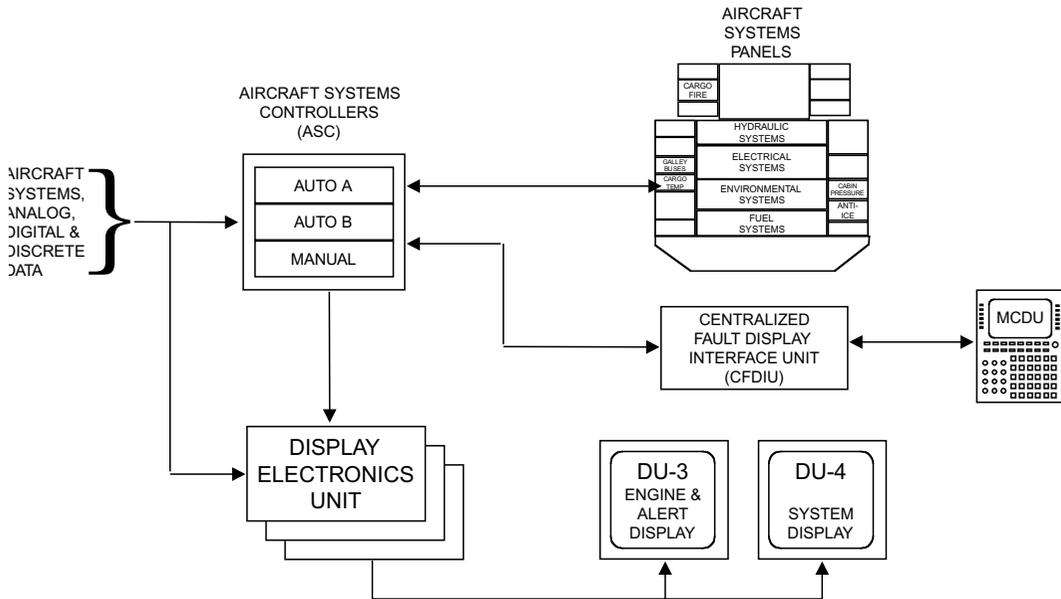
**FIGURE 31.10** Generalized architecture for aircraft system controllers (ASC).
