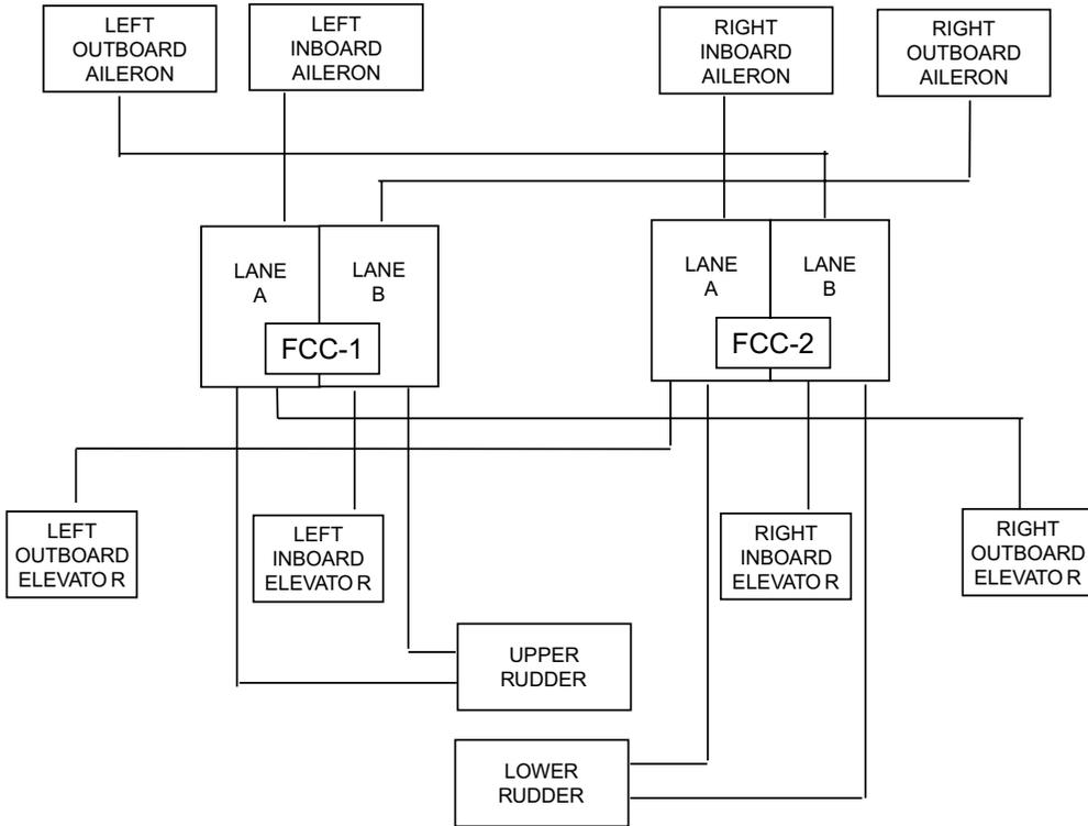
FIGURE 31.3 AFS actuator architecture.
