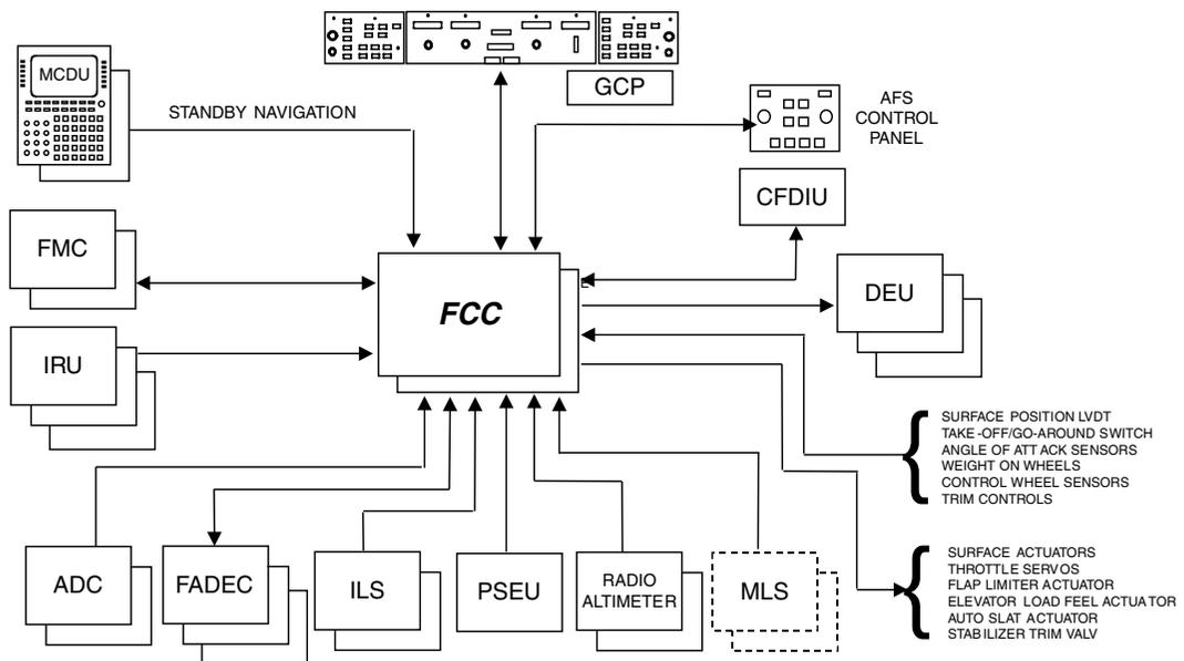
**FIGURE 31.2** Auto Flight System (AFS) architecture.
