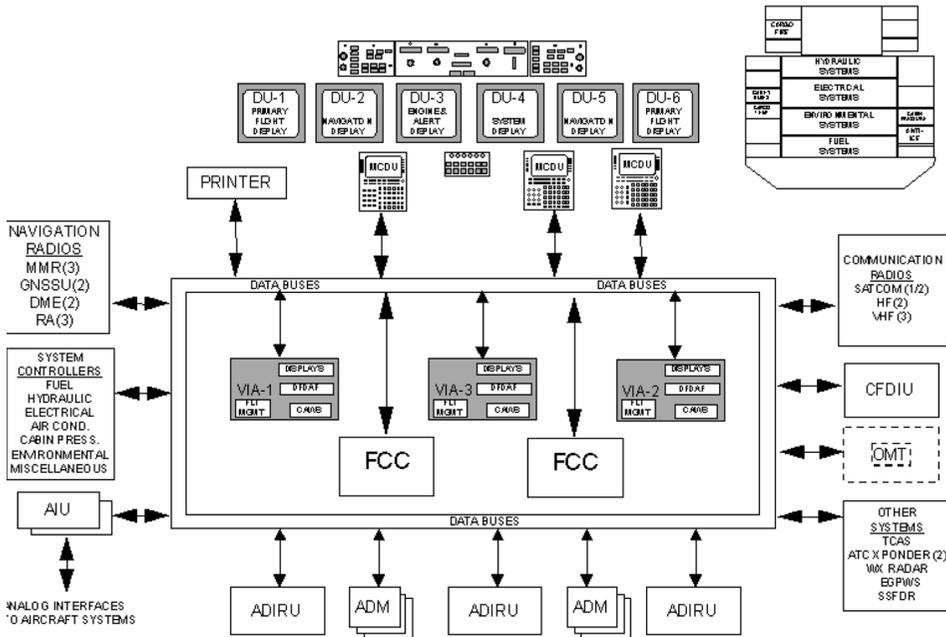
FIGURE 31.12 Advanced common flight deck (ACF) architecture.
