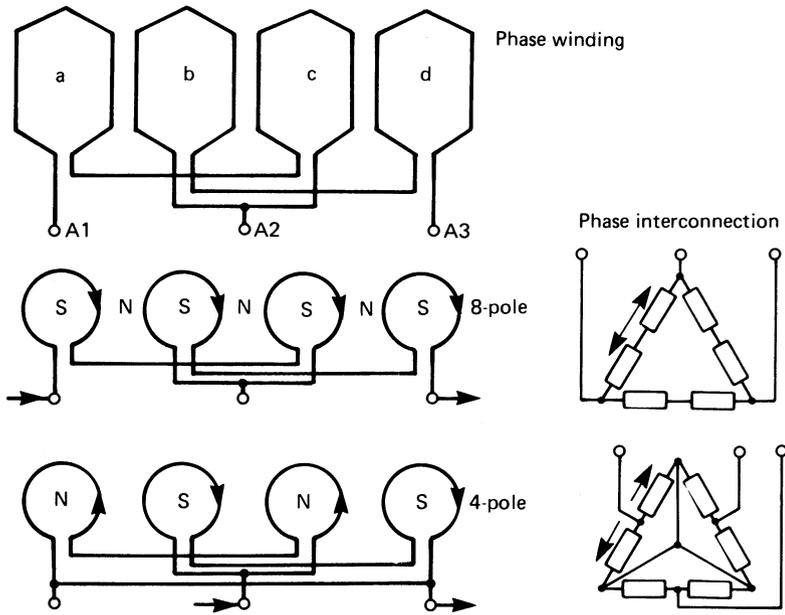
Figure 20.40 Pole change in the ratio 2:1
