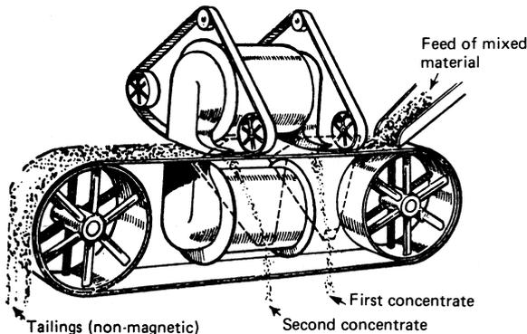
Figure 20.11 Wetherill separator
