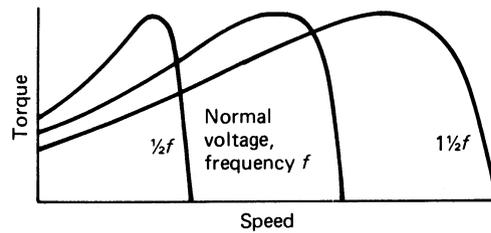
Figure 20.42 Torque-speed relationships for variable frequency
