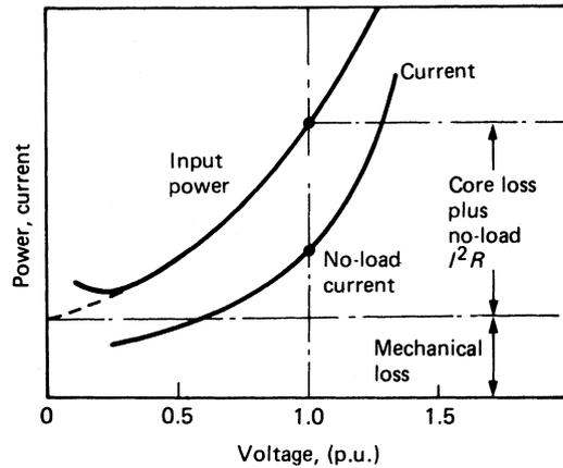
Figure 20.57 Induction motor: no-load characteristics
