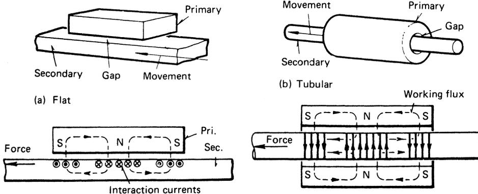
Figure 20.60 Linear motors: (a) flat; (b) tubular
