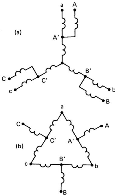
Figure 20.41 Pole-amplitude modulation. Unmodulated/modulated connections: (a) parallel-Y/series-Y; (b) parallel-Y/series-delta. Poles  $2p$ : supply to ABC with abc joined. Poles  $2(p \pm 4)$ : supply to abc with ABC isolated
