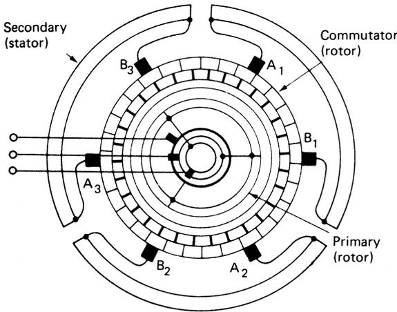
Figure 20.45 Schrage motor; stator and rotor circuits
