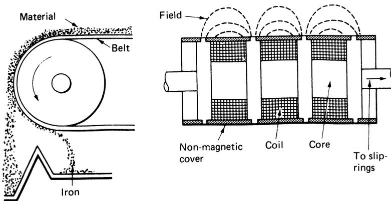
Figure 20.9 Magnetic pulley separator
