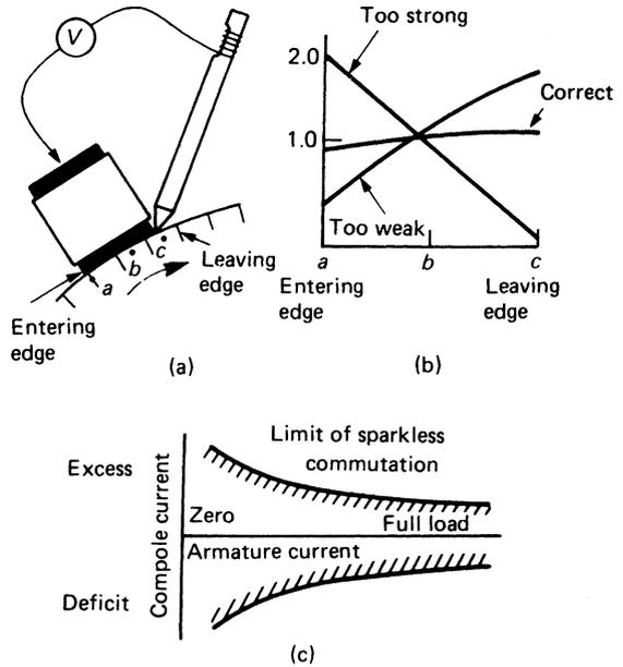
Figure 20.56 Commutation tests
