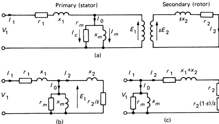
Figure 20.37 Three-phase induction motor: equivalent circuit per phase
