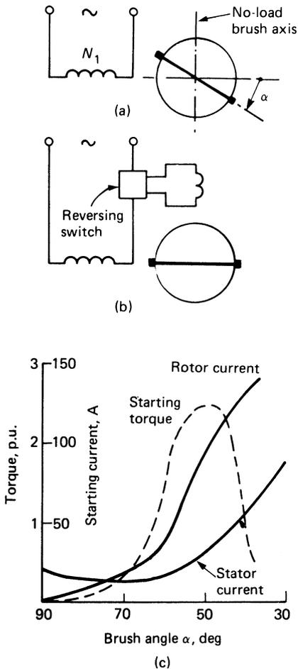
Figure 20.50 Repulsion motor: alternative forms and starting characteristics
