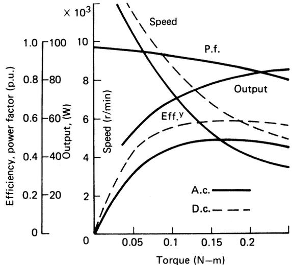
**Figure 20.49** Characteristics of a 75 W universal motor
