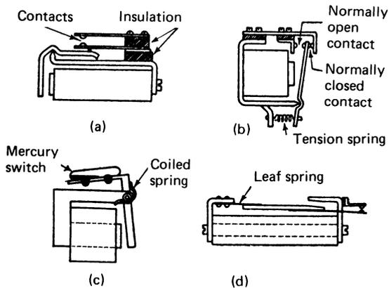
Figure 20.18 Electromagnetic relays
