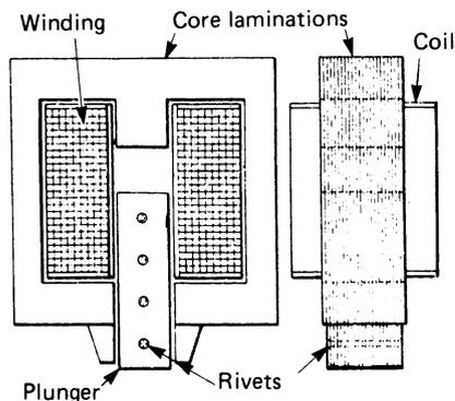
Figure 20.6 Single-phase actuator
