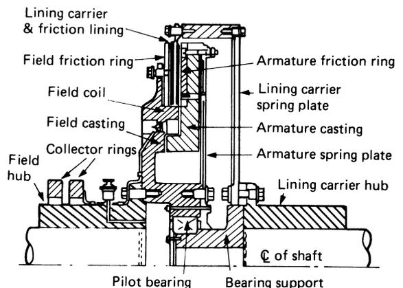
Figure 20.12 Electromagnetic clutch with double friction lining
