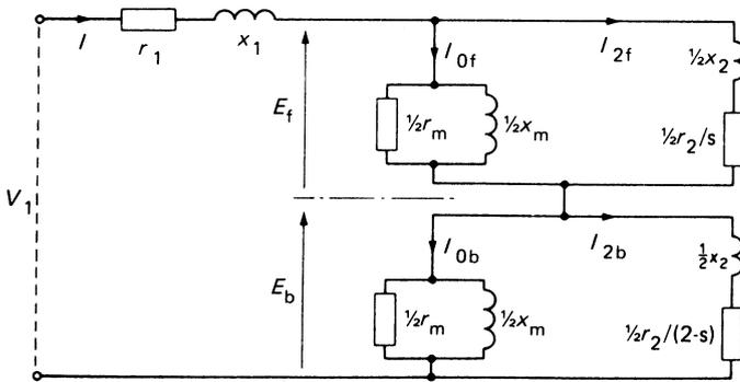
Figure 20.52 Simple one-phase induction motor: equivalent circuit
