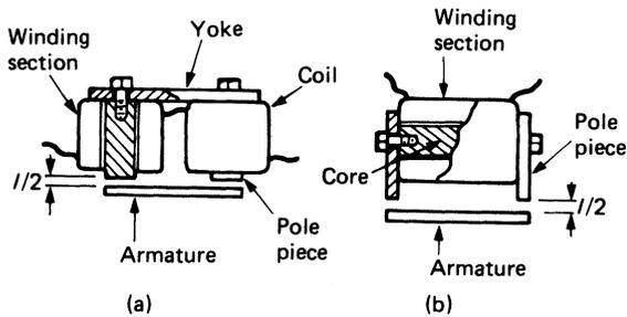
Figure 20.3 Tractive electromagnets
