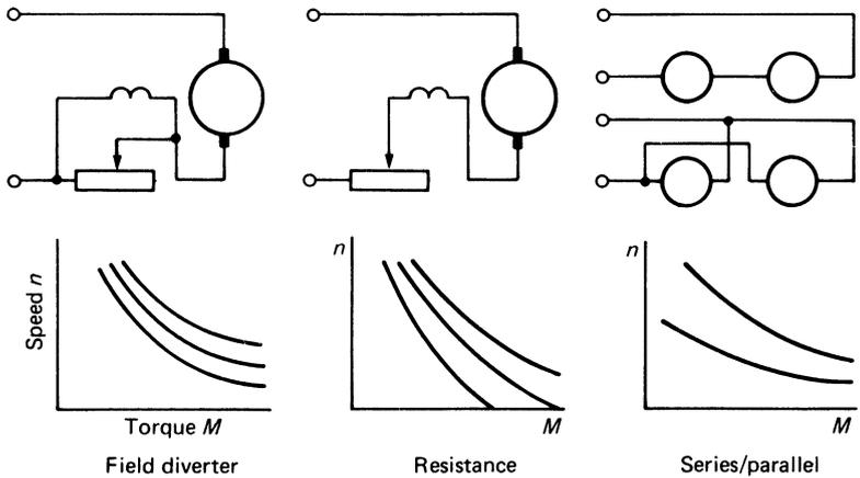
Figure 20.31 Series motor: speed control
