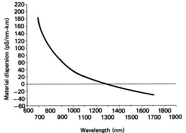
Figure 37.6 Material dispersion versus wavelength for silica
