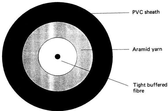
Figure 37.8 Single-fibre cable
