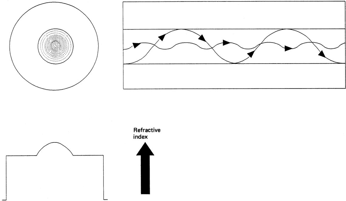
Figure 37.5 Typical ray paths for graded index fibre
