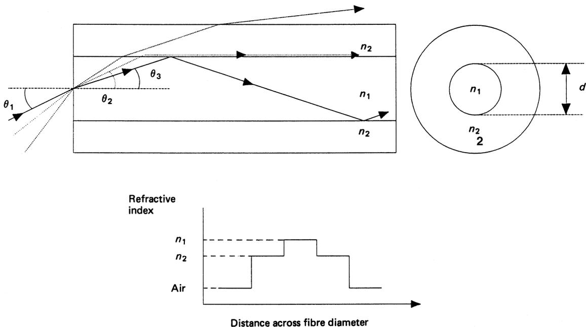
Figure 37.1 Ray diagram for multimode step index fibre
