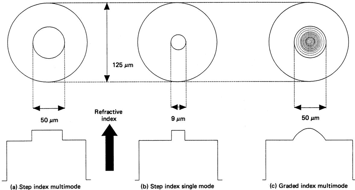
Figure 37.4 Refractive index profiles (typical dimensions shown)
